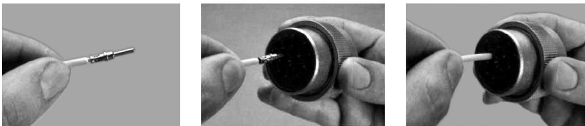
Figure 7-14. HD/HDP Contact Installation
